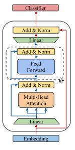
Figure 4: Illustration of MobileBERT<sub>TINY</sub>. red lines denote inter-block flows while blue lines intra-block flows.
